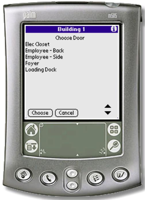
5. If you have communicated with this controller hardware before, or you just selected the door from the list in the step above, then LS Link will ask you to verify the door controller you are communicating with.
