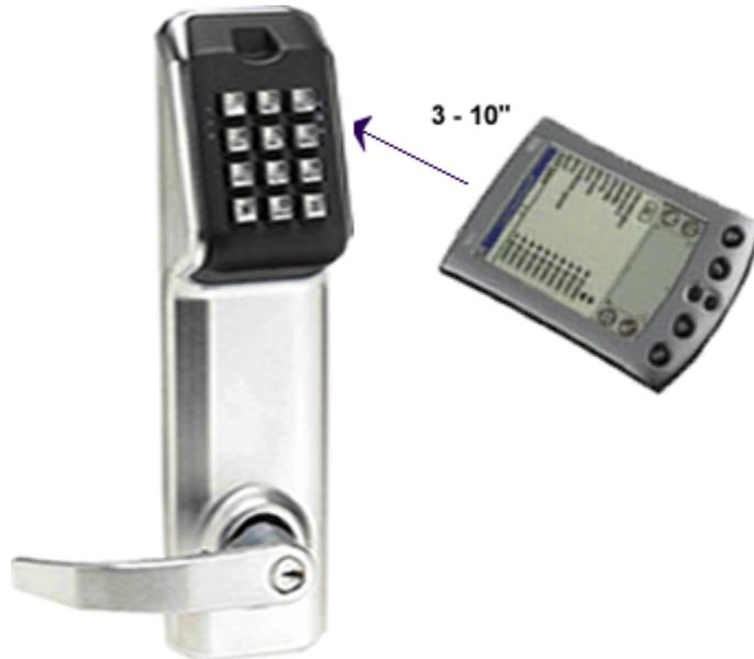
**NOTE:** The optimal distance between the PDA and the controller is approximately 3" to 10". Some PDA's perform better at the shorter range and some perform better at the longer range due to the variations in the infrared lens of the PDA hardware. Longer export and import times will result from putting the PDA either too close or too far away from the infrared receiver of the controller. This extra time is due to retries that may result from communication errors.
